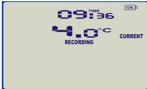
The display shows the current temperature, current time, battery status and any alarm triggers and is updated each time a log is taken.
