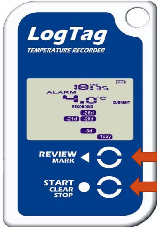
Start/Stop/Clear button functions require the button to be pressed continuously for 4 seconds and then released when the related flashing indicator stops flashing.
