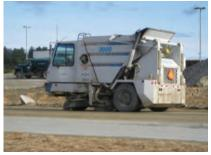
**Sweep and Vacuum** paved road surface when dry. Sweep from the center line to the edge of the travel way. Do not sweep into a waterbody or wetland. The public roadway may also require sweeping.
