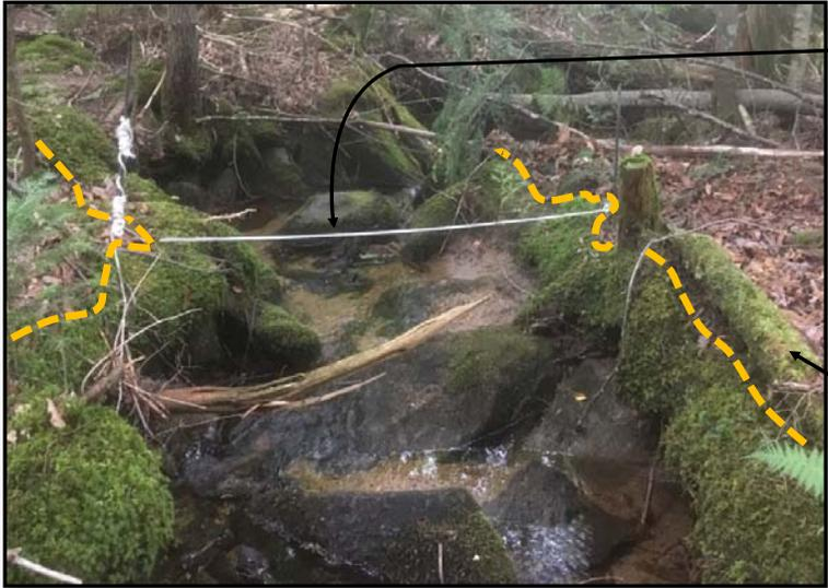
Staked line for measuring width and depth.
