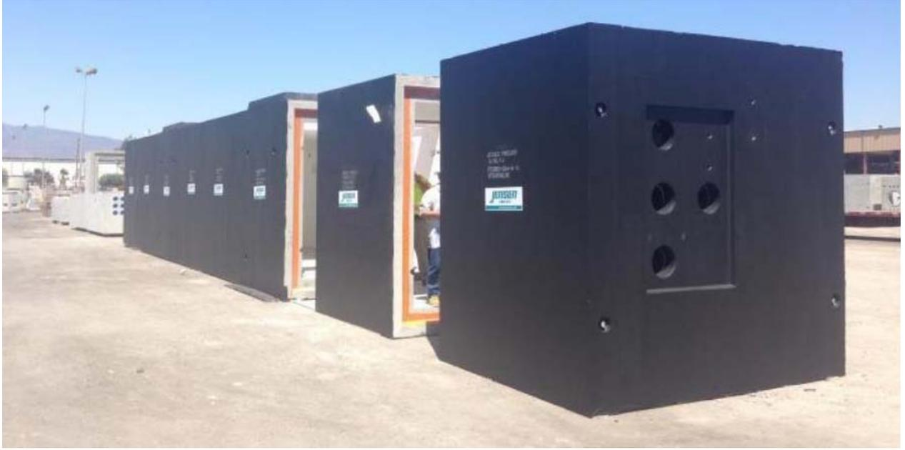
*Figure 3 - 500kV Splicing Vault*
