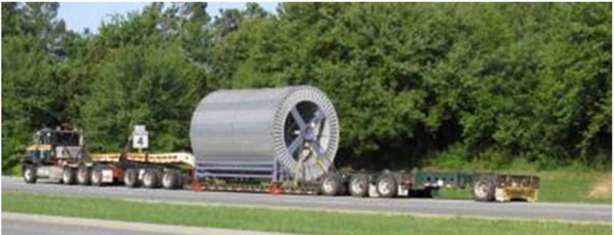
*Figure 10- Oversized Reel Transport, 4,724 feet of 230kV Cable*
